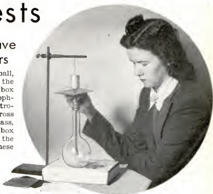
An insulating plate inserted between the charged box and the electroscope increases inductive effect across the air space
